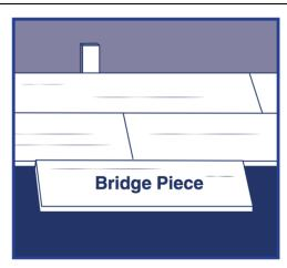
Step 6: Attach a scrap piece of floor to bridge the gap between ends of planks.
