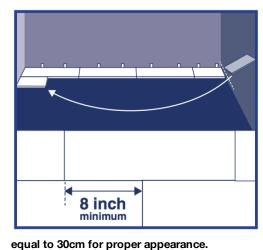
leftover flooring from first row as starter for second row. There must be at least 20cm between flooring end joints on adjacent rows. FOR TILE INSTALLATIONS: The distance between end joints should be
